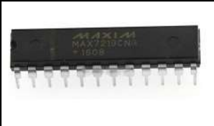
MAX7219 MAX7219CNG MAX7219ENG DIP24 In-line display driver
